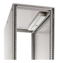
**Description:** Fluorescent lamp equipped with switch, integrated socket and a protection cap. A male connector is provided for connection to the power on one side and by a pass-through circuit to a female connector allows a further connection on the other side. An additional connector allows the activation of the lamp by a door switch.
