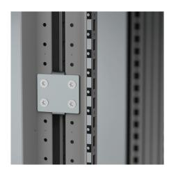
**Descripción:** Brackets mounted on the outside hole pattern of the frame ensuring a strong and 3 dimensional alignment of the mild steel bayed enclosures with an "auto spacer" function. This method of baying enclosures also has the advantage of creating a direct earthing connection between the enclosure frames.
