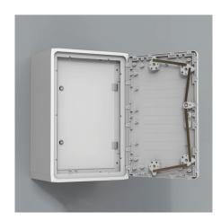
**Description:** For controls, meters, lamps, etc. Hinges can be mounted to allow left or right hand opening. Lock double-bit 3 mm insert. Distance between UID and enclosure door: 48 mm.
