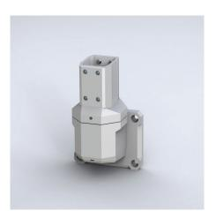
**Description:** Wall joint with vertical outlet component for SL system, angle of rotation 300° with stop. Rotation angle limiter is to be ordered as a separate product. Cable access with a plastic click-in cover.
