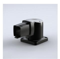
**Description:** Set-up joint component for SM system, angle of rotation 300° with stop. Rotation angle limiter is to be ordered as a separate product. Cable access with a plastic screw fitted cover.
