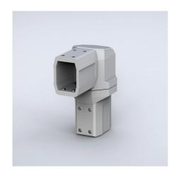
**Description:** Rotary elbow component for SL system, angle of rotation 300° with stop. Rotation angle limiter is to be ordered as a separate product. Cable access with a plastic click-in cover.
