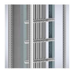
**Description:** Busbar supports up to 1600A to be mounted vertically behind the plug-in compartments. Rated short-time withstand current up to 35KA with rear supports and up to 50KA with rear and front supports. Mounts to the vertical profiles included in the rear cover plate for plugin sections MSSB.
