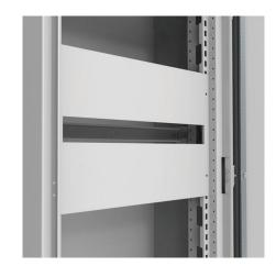
**Description:** Slotted front panel for modular assemblies. Provided with one DIN rail per row for modular components. It has a top and bottom bending to provide extra rigidity.
