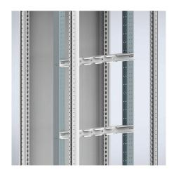
**Description:** Busbar supports up to 1600A to be mounted vertically behind the fixed compartments. Mounts to the vertical profiles MSFP. Rated short-time with stand current up to 35 kA with rear supports and up to 50 kA with rear and front supports.
