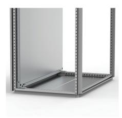
**Description:** Creates an installation surface over the full width of the enclosure. Easy installation by use of sliding profiles MTS from the side. Nominal width equals the enclosure width. When combining enclosures the MPWs can be connected and slid in as one installation surface. Can not be mounted in the rearmost position.
