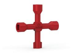
**Description:** Multi-Key function with nVent HOFFMAN logo and a different key in every end: double-bit 5 mm, square 8 mm, triangle 8 mm and a standard hexagonal adaptor to use with the screw ends.
