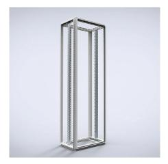
**Description:** Vertical profiles with 25 mm hole pattern, to support DIN rails and appropriate telequick mounting plates. Adjustable in depth in steps of 25 mm.
