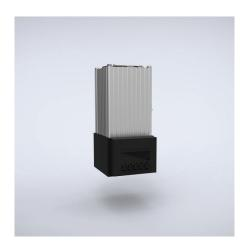
**Description:** Heater with fan to be fixed as desired, but preferably in vertical position to prevent condensation. The fan assists the natural convection for fast distribution of the heat in large enclosures. Mounting clip for 35 mm DIN rail (EN60715).
