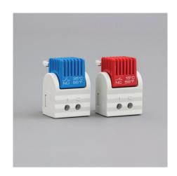
**Description:** Pre-set thermostats to manage temperature in panels. Sensor element thermostatic bimetal. Red one (EFR202) with a normally closed contact for regulating heaters. Blue one (EFR201) with a normally opened contact for regulating cooling devices or signal devices. Mounting clip for 35 mm DIN rail (EN 60715).
