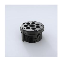
**Description:** Round plastic cable entry for a fast, economical and tool-free incoming of cables and/or pneumatic conduits inside the enclosure. Integrated seal. For snap-in mounting. Snap-in system works at wall thicknesses of 1.4 to 2 mm. Installation height: 9 mm outside, and 24-25 inside.
