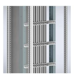
**Beschreibung:** Busbar supports up to 1600A to be mounted vertically behind the plug-in compartments. Rated short-time withstand current up to 35KA with rear supports and up to 50KA with rear and front supports. Mounts to the vertical profiles included in the rear cover plate for plugin sections MSSB.
