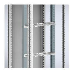
**Beschreibung:** Busbar supports up to 1600A to be mounted vertically behind the fixed compartments. Mounts to the vertical profiles MSFP. Rated short-time withstand current up to 35 kA with rear supports and up to 50 kA with rear and front supports.
