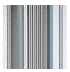
**Beschreibung:** Vertical busbar to build up the plug-in system. The MSBS bars are fixed in the MSVH supports with standard bolts, washers and nuts. The rated current can be increased up to  $2 \times 1400A$  if the incoming connetion is in the middle.
