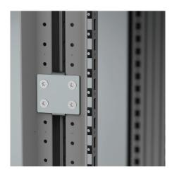
**Beschreibung:** Brackets mounted on the outside hole pattern of the frame ensuring a strong and 3 dimensional alignment of the mild steel bayed enclosures with an "auto spacer" function. This method of baying enclosures also has the advantage of creating a direct earthing connection between the enclosure frames.
