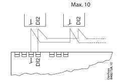
The following controllers can be connected up in this way: EKC 204A, AK-CC 210, AK-CC 250, AK-CC 450, AK-CC 460, AK-CC 550,
