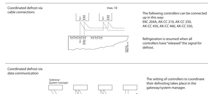
Refrigeration is resumed when all controllers have "released" the signal for defrost.
