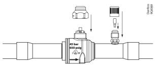
Install Schrader valve with approx. torque 0.3 Nm / 0.2 ft-lbs
