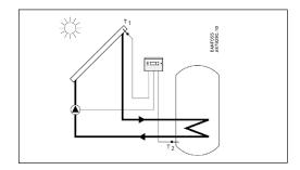
T1: Temperature sensor in solar collector
