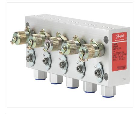
The pressure test valve, type MBV 5000 is a part of the block concept which has been developed to save space, weight and costs. The test valve is intended for use in many applications, for example monitoring, alarm indication, shut-down, diagnosing on equipment such as motors, gears, thrusters, pumps, filters, compressors etc.
