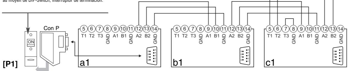
[P1]-Terminate the first WM14 "a1" positioning the dip-switch in ON on the "Con P" connector and the last WM14 "c1" by connecting T1, T2, T3. Use a two pole shielded cable, about the connection length (from the first to the last instrument) refer to "TAB1".
