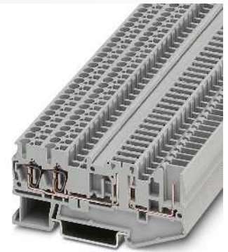
2,5 (4) mm 2 , 20 A, Trennklemme, 3 Anschlüsse
