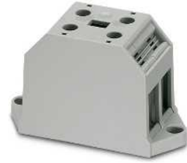
35 (35) mm 2 , 125 A, Klemmenblock, 2-polig, intern verbunden
