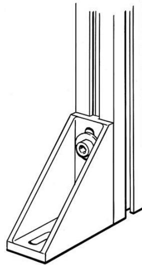
Plancher support en aluminium. Dimension 42x100x100mm, pré-monté.
