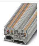
Disconnect terminal block, Connection type: Push-in connection, Cross section: 0.14 mm² - 4 mm², AWG: 26 - 12, Nominal current: 20 A, Nominal voltage: 400 V, Length: 67.8 mm, Width: 5.2 mm, Color: gray, Assembly: NS 35/7,5, NS 35/15
