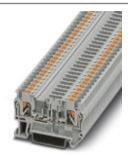
Disconnect terminal block, Connection type: Push-in connection, Cross section: 0.14 mm² - 4 mm², AWG: 26 - 12, Nominal current: 20 A, Nominal voltage: 400 V, Length: 56 mm, Width: 5.2 mm, Color: gray, Assembly: NS 35/7,5, NS 35/15
