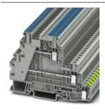
Ground modular terminal block, Connection method: Screw connection, Cross section: 0.14 mm<sup>2</sup> - 6 mm<sup>2</sup>, AWG: 26 - 10, Width: 6.2 mm, Height: 60.1 mm, Color: gray, Mounting type: NS 35/7,5, NS 35/15
