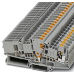
Test disconnect terminal block, Connection method: Push-in connection, Cross section: 0.5 mm 2 -10 mm 2 , AWG: 20 - 10, Width: 8.2 mm, Color: gray
