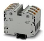
High-current terminal block, Connection method: Power-Turn connection, Cross section: 2.5 mm² - 35 mm², AWG: 12 - 2, Width: 48 mm, Color: gray, Mounting type: NS 35/15
