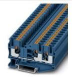
Feed-through terminal block, Connection method: Push-in connection, Cross section: 0.5 mm<sup>2</sup> - 10 mm<sup>2</sup>, AWG: 20 - 8, Width: 8.2 mm, Height: 42.2 mm, Color: gray, Mounting type: NS 35/7,5, NS 35/15
