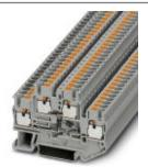
Double-level terminal block, with integrated diode, Cross section: 0.14 mm² - 4 mm², AWG: 26 - 12, Connection type: Push-in connection, Width: 5.2 mm, Color: gray, Mounting type: NS 35/7,5, NS 35/15
