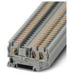
Feed-through terminal block, Connection method: Push-in connection, Cross section: 0.2 mm<sup>2</sup> - 6 mm<sup>2</sup>, AWG: 24 - 10, Width: 6.2 mm, Color: black, Mounting type: NS 35/7,5, NS 35/15
