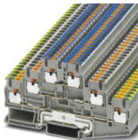
Ground modular terminal block, Connection method: Push-in connection, Cross section: 0.14 mm 2 - 4 mm 2 , AWG: 26 - 12, Width: 5.2 mm, Color: gray, Mounting type: NS 35/7,5, NS 35/15
