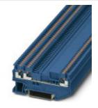
Feed-through terminal block, same shape as disconnect terminal block, Connection method: Push-in connection, Cross section: 0.14 mm<sup>2</sup> - 1.5 mm<sup>2</sup>, AWG: 26 - 14, Width: 3.5 mm, Height: 30.5 mm, Color: blue, Mounting type: NS 35/7,5, NS 35/15
