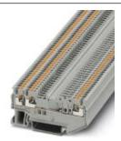
Disconnect terminal block, Connection type: Push-in connection, Cross section: 0.14 mm² - 1.5 mm², AWG: 26 - 14, Nominal current: 10 A, Nominal voltage: 400 V, Length: 67.8 mm, Width: 3.5 mm, Color: gray, Assembly: NS 35/7,5, NS 35/15
