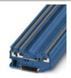
Disconnect terminal block, Connection type: Push-in connection, Cross section: 0.14 mm<sup>2</sup> - 1.5 mm<sup>2</sup>, AWG: 26 - 14, Nominal current: 10 A, Nominal voltage: 400 V, Length: 67.8 mm, Width: 3.5 mm, Color: blue, Assembly: NS 35/7,5, NS 35/15
