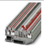
Knife disconnect terminal block, With red disconnect knife and red actuation triggers, Connection type: Pushin connection, Cross section: 0.14 mm<sup>2</sup> - 4 mm<sup>2</sup>, AWG: 26 - 12, Nominal current: 20 A, Nominal voltage: 400 V, Length: 74 mm, Width: 5.2 mm, Color: gray, Assembly: NS 35/7,5, NS 35/15
