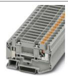
Feed-through terminal block, Connection type: Push-in connection, Screw connection, Cross section: 0.5 mm<sup>2</sup> - 10 mm<sup>2</sup>, AWG :20- 10, Width: 8.2 mm, Color: gray, Mounting: NS 35/7,5, NS 35/15
