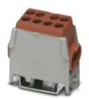
Trunk line branch terminal, Connection method: Screw connection, Number of positions: 1, Cross section: 1.5 mm² - 25 mm², AWG: 8 - 2, Width: 23 mm, Color: brown, Mounting type: NS 35/7,5, NS 35/15
