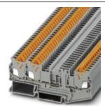
Disconnect terminal block, Connection method: Quick connection, Cross section: 0.25 mm² - 1.5 mm², AWG: 24 - 16, Width: 5.2 mm, Height: 39.3 mm, Color: gray, Mounting type: NS 35/7,5, NS 35/15
