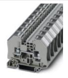
Feed-through terminal block with bolt connection technology and transparent safety contact hood, cross section: 0.1 - 6 mm<sup>2</sup>, AWG: 26 - 10, width 16.3 mm, color: gray
