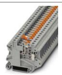
Knife disconnect terminal block, Connection type: Screw connection, Cross section: 0.14 mm² - 6 mm², AWG: 26 - 10, Nominal current: 20 A, Nominal voltage: 500 V, Length: 57.8 mm, Width: 6.2 mm, Color: gray, Assembly: NS 35/7,5, NS 35/15
