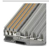
Feed-through terminal block, Connection method: Push-in / plug connection, Cross section: 0.14 mm<sup>2</sup> - 4 mm<sup>2</sup>, AWG: 26 - 12, Width: 5.2 mm, Height: 35.3 mm, Color: gray, Mounting type: NS 35/7,5, NS 35/15
