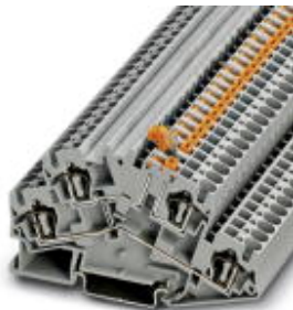
Knife disconnect terminal block, Cross section: 0.08 mm 2 - 6 mm 2 , AWG: 28 - 10, Connection type: Spring-cage connection, Width: 6.2 mm, Color: gray, Mounting type: NS 35/7,5, NS 35/15
