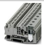
Feed-through terminal block, Connection method: Spring-cage connection, Cross section: 0.2 mm<sup>2</sup> - 10 mm<sup>2</sup>, AWG: 24 - 8, Width: 16.2 mm, Color: blue, Mounting type: NS 35/7,5, NS 35/15
