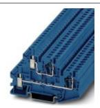
Feed-through terminal block, Connection method: Spring-cage connection, Cross section: 0.08 mm² - 6 mm², AWG: 28 - 10, Width: 6.2 mm, Color: blue, Mounting type: NS 35/7,5, NS 35/15
