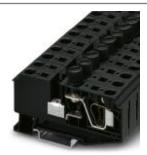
Spring-cage terminal block-fuse terminal block for cartridge fuse inserts with screw cap, cross section: 0.5 - 6 mm², width: 12 mm, color: black
